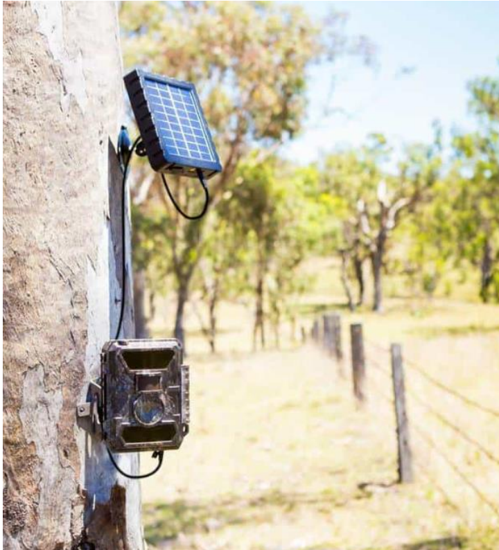
Figure 5 Wildlife Camera and Solar Panel Example Mounting Configuration
