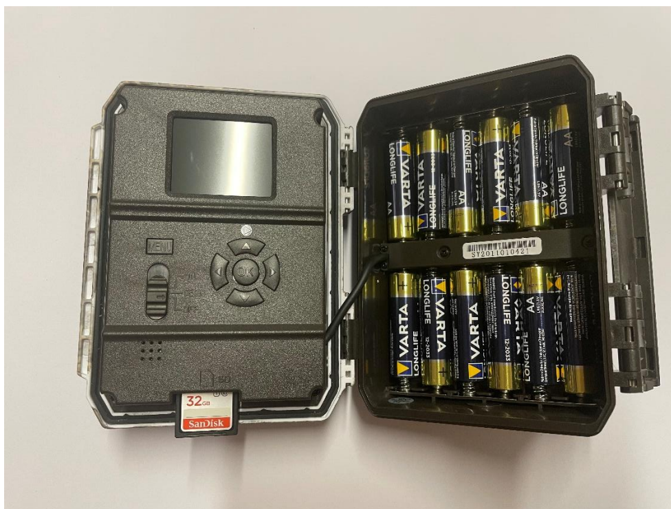
Figure 2 Swift Enduro Wildlife Camera Inside View
